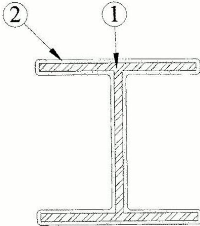
1. **Steel Column** — Wide flange steel columns with the minimum sizes shown in the tables below. Columns shall be free of dirt, loose scale and oil. Column shall be primed with 0.003 in. dry film thickness of modified alkyd, epoxy, organic zinc or inorganic zinc based primer.
