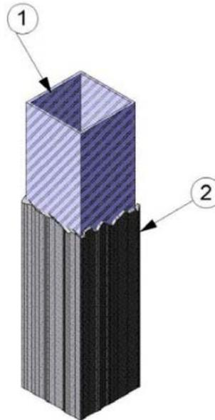
**1. HOLLOW STRUCTURAL STEEL COLUMN:** Use hollow steel sections, rectangular-shape (shown) or circular-shape (not shown), having nominal  $H_p/A$  or  $W/D$ , or  $A/P$  section factors based on four-sided exposure. Refer to Table CC/IF 180-03 for specific application thickness of intumescent mastic fireproofing (Item 2) based on nominal  $H_p/A$ ,  $W/D$ , or  $A/P$  section factors.
