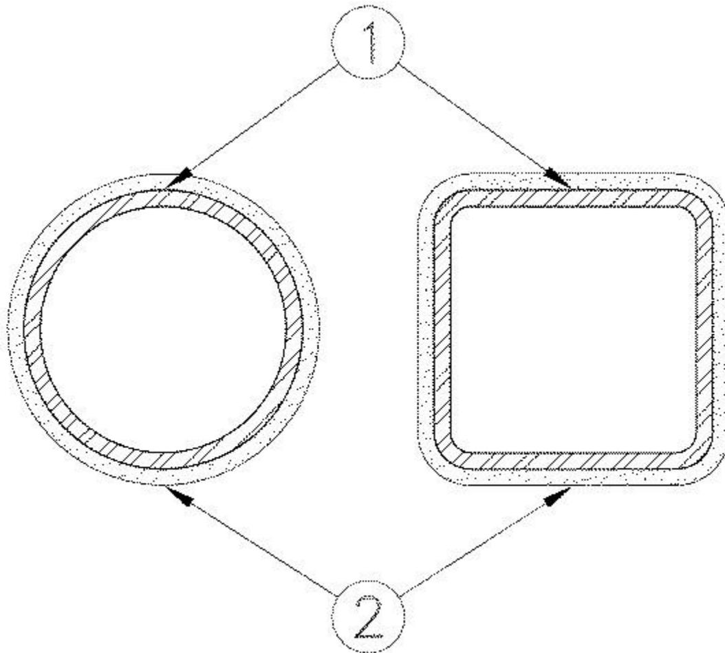
1. **Steel Column** — Square, rectangular or circular tubular steel columns with the minimum sizes shown in the table below. Steel columns shall be free of dirt, loose scale and oil. Column shall be primed with metal alkyd primer.
