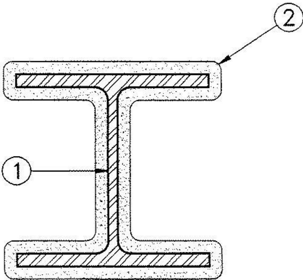
**1. Steel Column** — Wide flange steel columns with the minimum sizes shown in the table below. Columns shall be free of dirt, loose scale and oil. Column shall be primed with metal alkyd primer.
