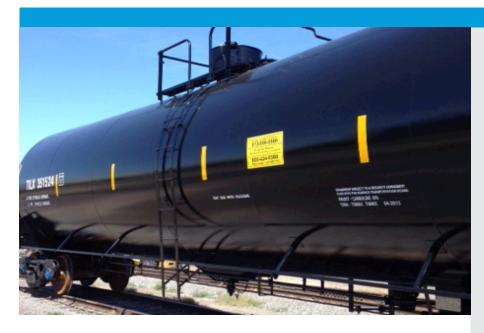
Plasite 4550 is a 100% solids reinforced novolac epoxy with excellent chemical resistance and quick return to service. It can withstand crude oil temperatures up to 350°F.
