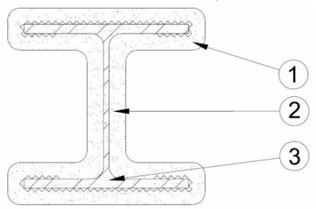
1. **Spray-Applied Fire-Resistive Materials\*** — See table below for appropriate thickness. Prepared by mixing with water according to instructions on each bag of mixture. Mixture can be spray or trowel applied in one or more coats to steel and mesh surfaces. Avg density of 40 pcf with min ind value of 37 pcf. For method of density determination, see Design Information Section, Sprayed Material. Surface of material may be lightly finished with a trowel.
