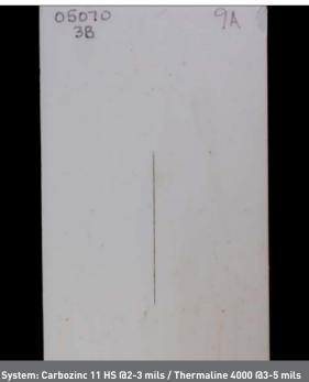
System: Carbozinc 11 HS @2-3 mils / Thermaline 4000 @3-5 mil Exposure: Salt Fog (ASTM B117); 5000 hours exposure
